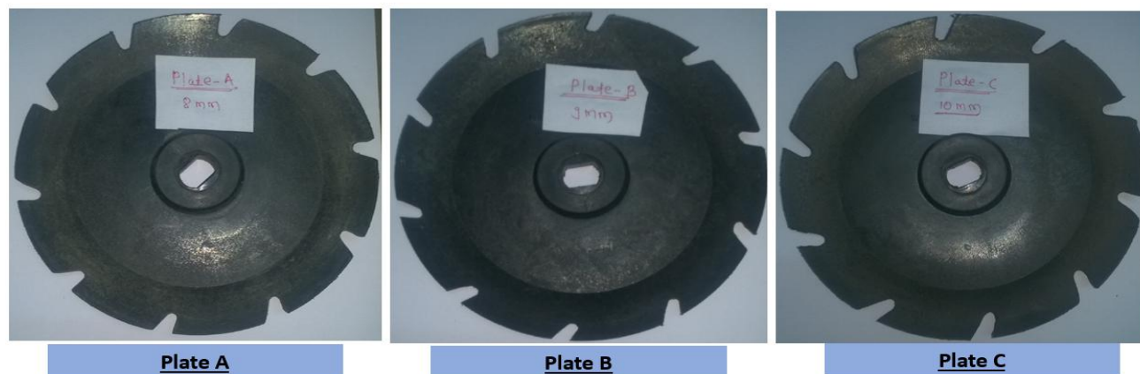
Fig.3 Metering plates used for metering of soaked okra seeds
