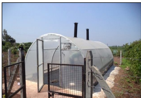
Fig 1: Schematic view of a solar tunnel dryer.
