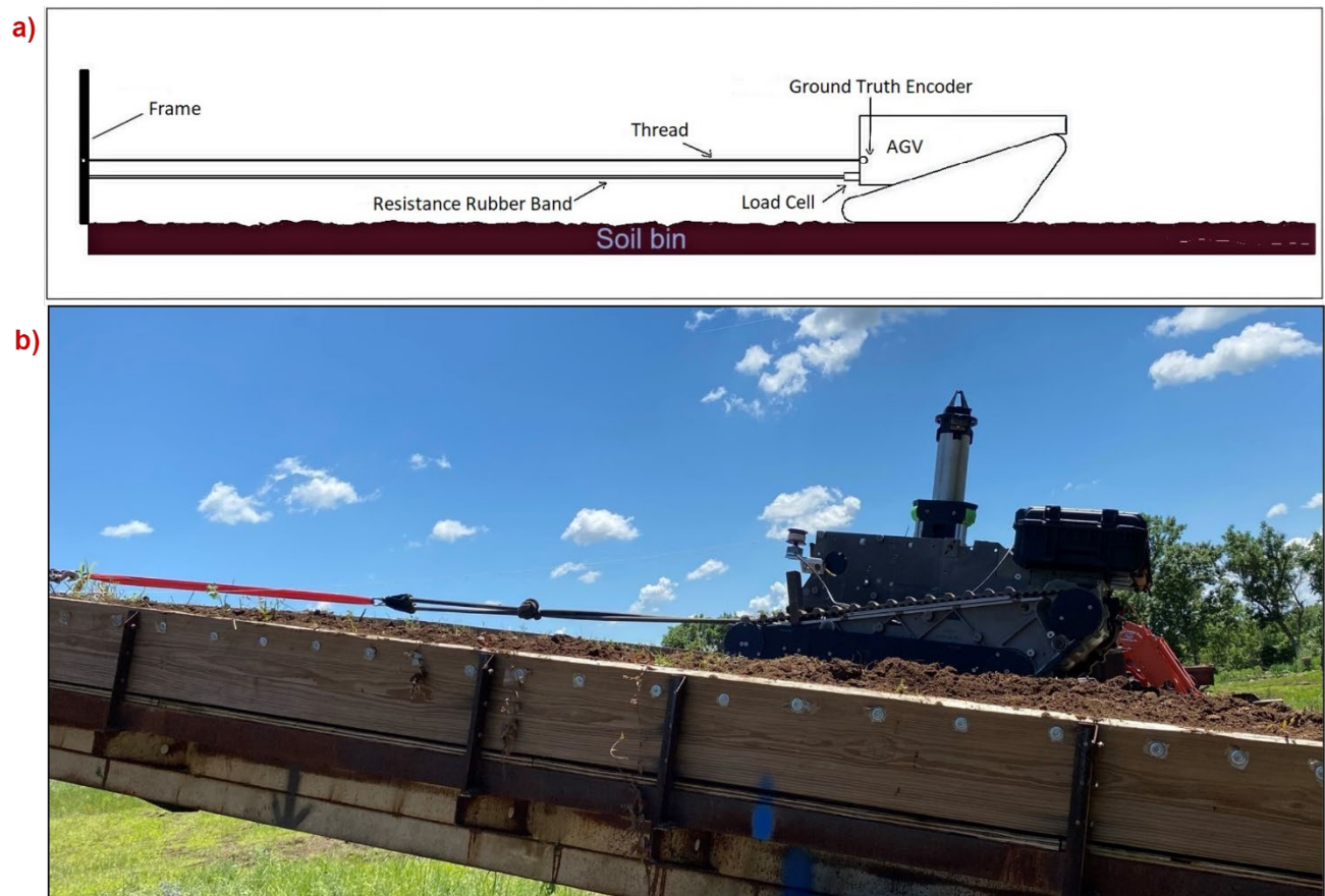
Figure 2. Drawbar pull test experimental setup: a) conceptual drawing, b) AGV operating on sloped soil bin. Direction of forward travel is from left to right.
